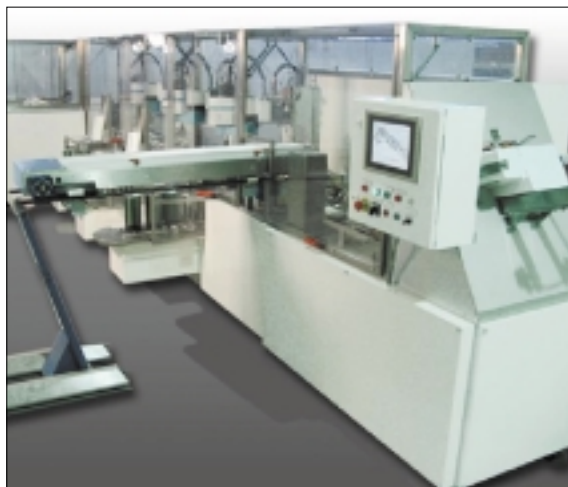
Stora Enso’s new DBS FF-80 automates packaging for its DVD version of the DBS Discbox Slider
